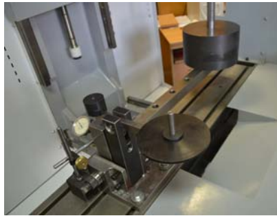
Fig. 12 Photo images of the device for measuring interface load capacity and compliance
